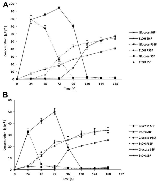
**Figure 1.** Profile of glucose (squares) and ethanol (triangle) during SHF (solid lines), PSSF (dash-dotted lines), and SSF (dotted lines) at 30%DM. Yeast was inoculated at 72, 24, and 0 h, respectively. The enzymes applied were CT2 (**Panel A**: scenarios A–C) and CN (**Panel B**: scenarios G–I), all at the high enzyme loading.
