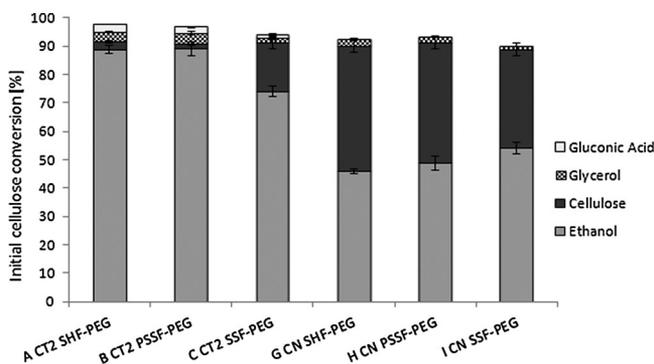
**Figure 8.** Final products yield as percentage of initial cellulose for scenarios A–C and G–I containing 1% of PEG3000. Scenarios A, B, and C represent SHF, PSSF, and SSF at 30% DM, respectively, applying CT2 at high enzyme loading. Scenarios G, H, and I represent SHF, PSSF, and SSF at 30% DM, respectively, applying CN at high enzyme loading.
