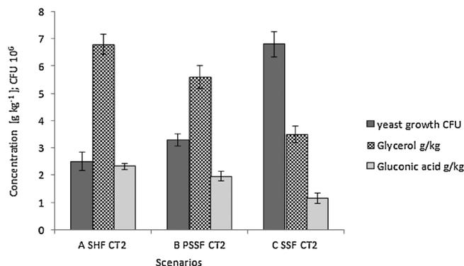
**Figure 6.** Final amount of gluconic acid, glycerol and yeast growth of scenarios A–C at 30%DM without PEG3000. Yeast growth represents the highest CFU-value during the process subtracted the CFU-value in the inoculum.
