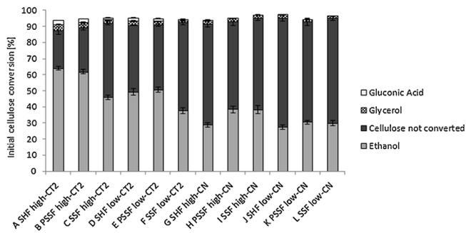
**Figure 2.** Final products yield as percentage of initial cellulose for all scenarios at 30%DM, after 168 h. Each bar represents the percentage of initial cellulose converted into the indicated products. Cellulose is the amount of fibers not hydrolyzed during the strategies as directly measured by compositional analysis. Gluconic acid, glycerol, and ethanol was measured and stoichiometric converted back to corresponding amount of cellulose. Ethanol includes the carbon dioxide.
