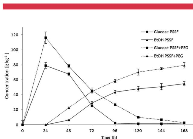
**Figure 7.** Concentration of glucose (squares) and ethanol (triangle) for scenario B at 30% DM comparing with PEG3000 (dashed lines) and without (solid lines). Time 24 h represent the yeast addition and temperature switch from 50 to 34°C.
