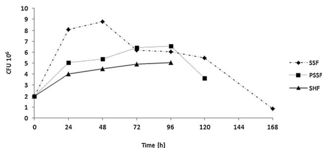
**Figure 5.** Cell viability in scenarios A–C, with CT2 at high enzyme loading, and 30% DM. Time 0 h represent the initial concentration of yeasts given by the inoculum.
