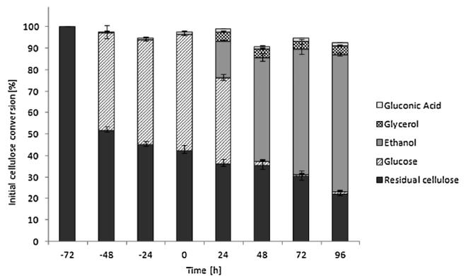
**Figure 3.** Product profiles as percentage of initial cellulose for scenario A, SHF with CT2 at high enzyme loading, and 30% DM. Time -72, -48, and -24 h represent the hydrolysis step at 50°C. Time 0 h represents onset of fermentation, that is, yeast addition and temperature change to the fermentation temperature of 34°C.
